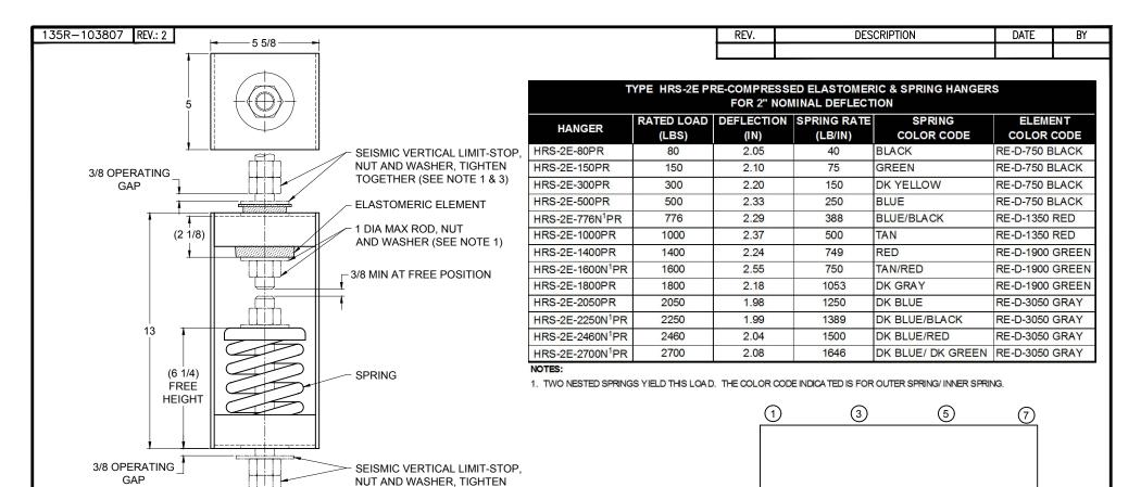
1. HANGER RODS, NUTS AND WASHERS, AS SHOWN. NOT BY THE VMC GROUP, INSTALL WASHER, 16 THK, MIN, X 3 O.D. MIN, WITH REQUIRED INSIDE DIAMETER TO ACCOMMODATE ROD SIZE IN USE. THIS CAN BE ACCOMPLISHED BY USING A SINGLE WASHER OR NOT MORE THAN TWO WASHERS.
